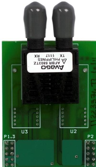
**Figure 1-8 Fiber optic Ethernet Board - ST Connector**
