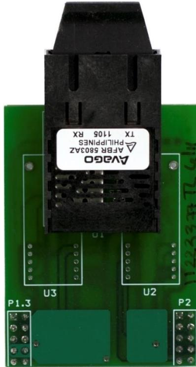
**Figure 1-7 Fiber optic Ethernet Board - SC Connector**
