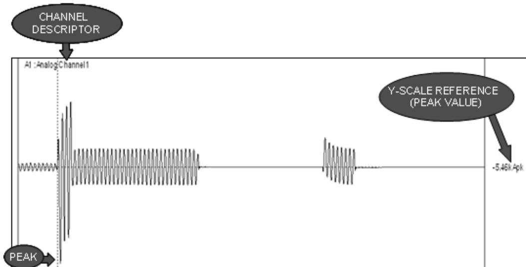
**Figure 2-36 Y-Scale – Optimized – Peak – Sample Printout**
