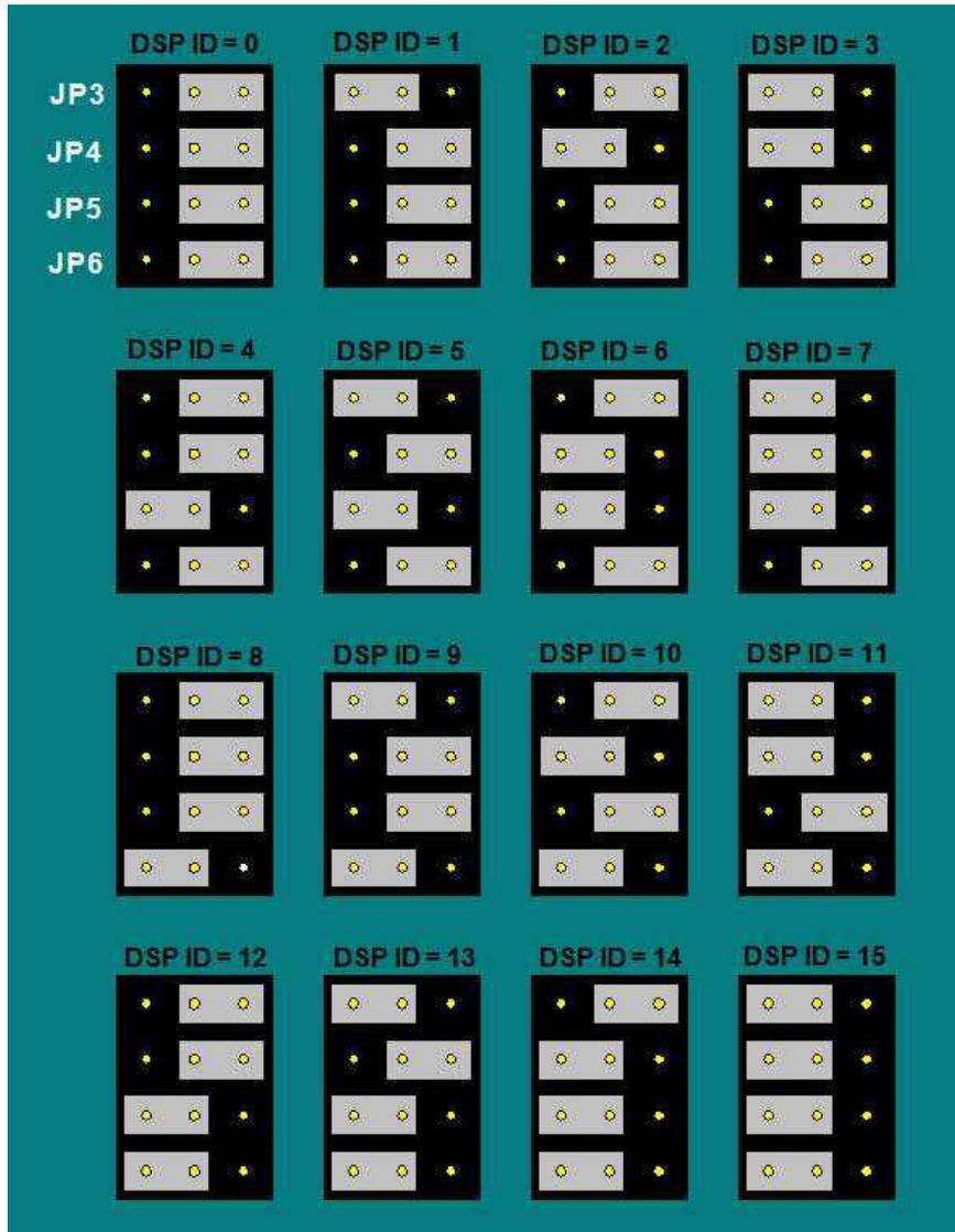
**Figure A.1.2-3 DSP Board Address Jumpers**
