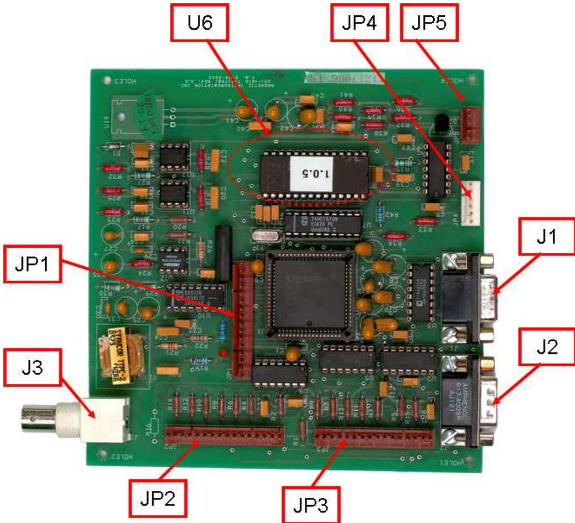
**Figure A.1.5-1 Input/Output Board (First Generation) – Modulated**
