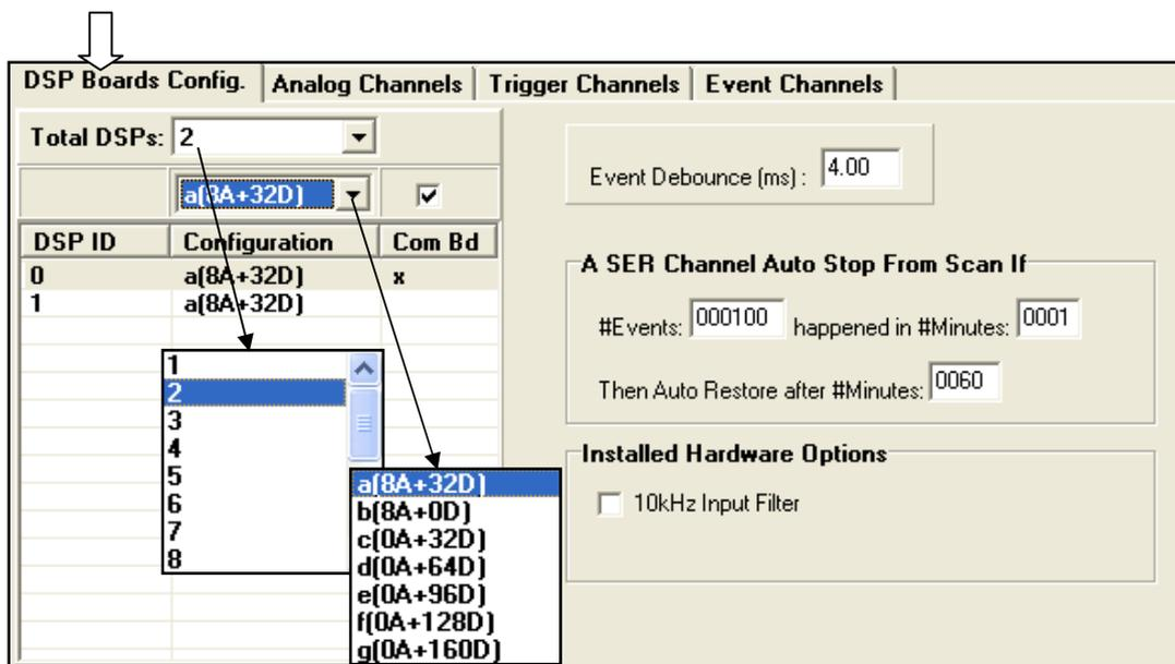
**Figure 2-77 DSP Boards Configuration Screen Tab – Version 2004**
