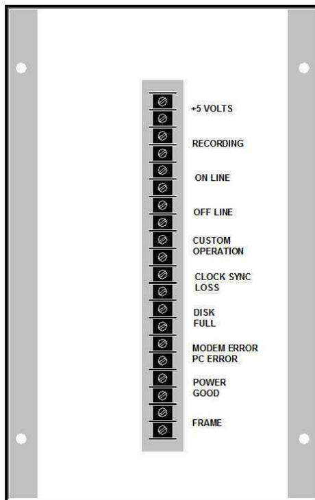
**Figure 1-11 Alarm Output Module**
