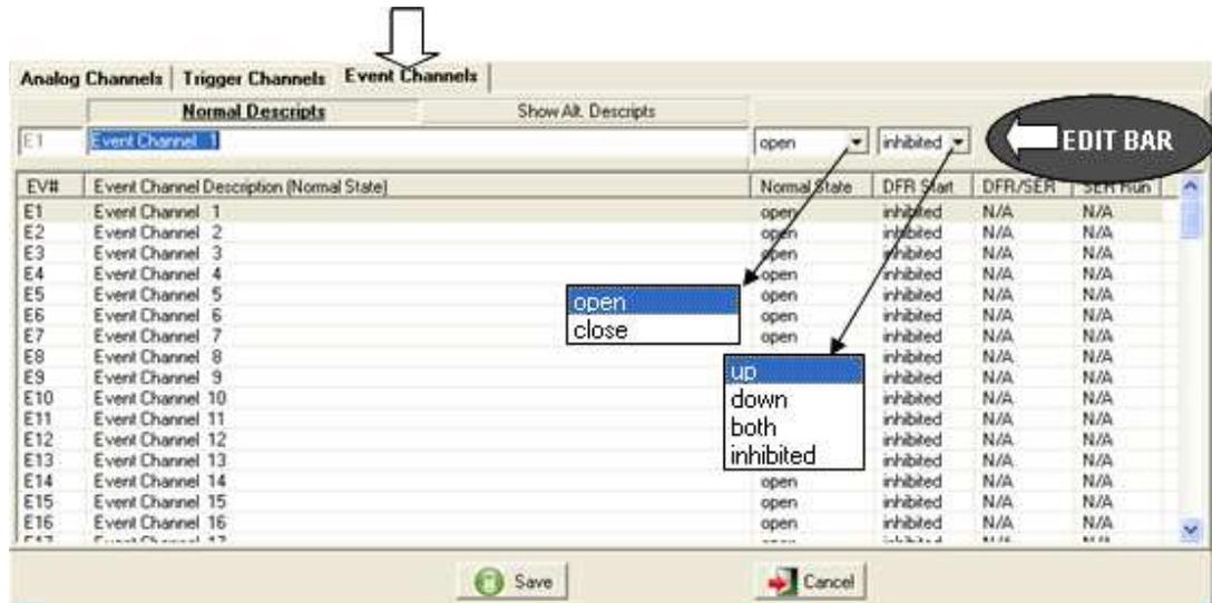
**Figure 2-75 Calibration Record Event Channels –Version 093a**
