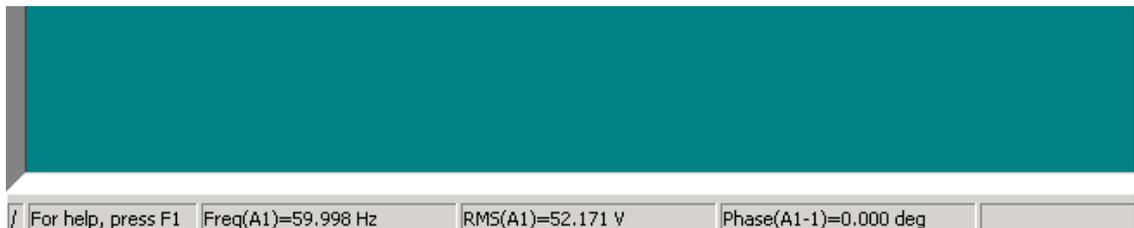
**Figure 2-28 WinDFR® Footer – Continuous Status Bar**
