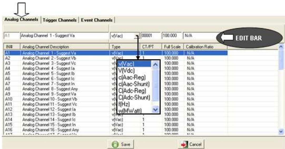
**Figure 2-73 Calibration Record Analog Channels –Version 093a**
