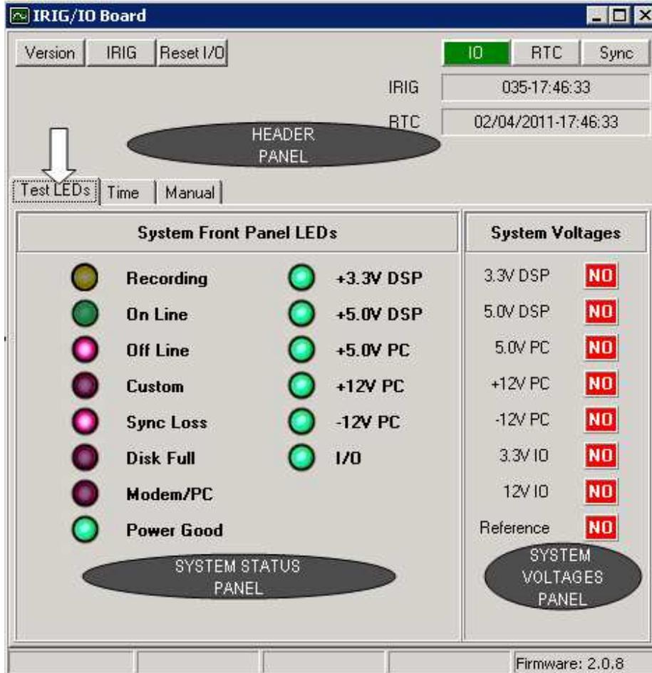
**Figure 3-5 I/O-IRIG Board Window**
