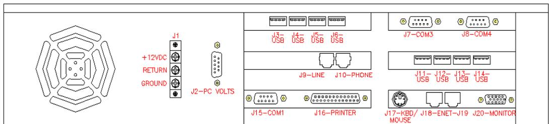
**Figure 1-6 DME Computer – Rear View**
