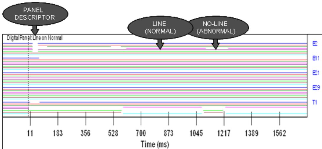
**Figure 2-44 All Events/Triggers – Line on Normal – Sample Printout**
