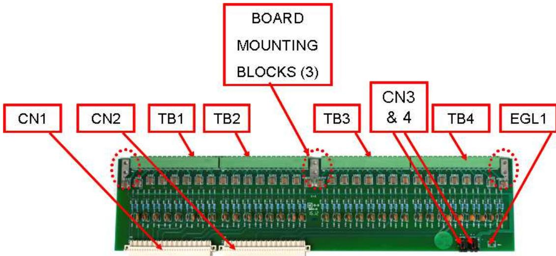
**Figure A.1.12 High-Voltage Digital Board (Single Board Assembly)**
