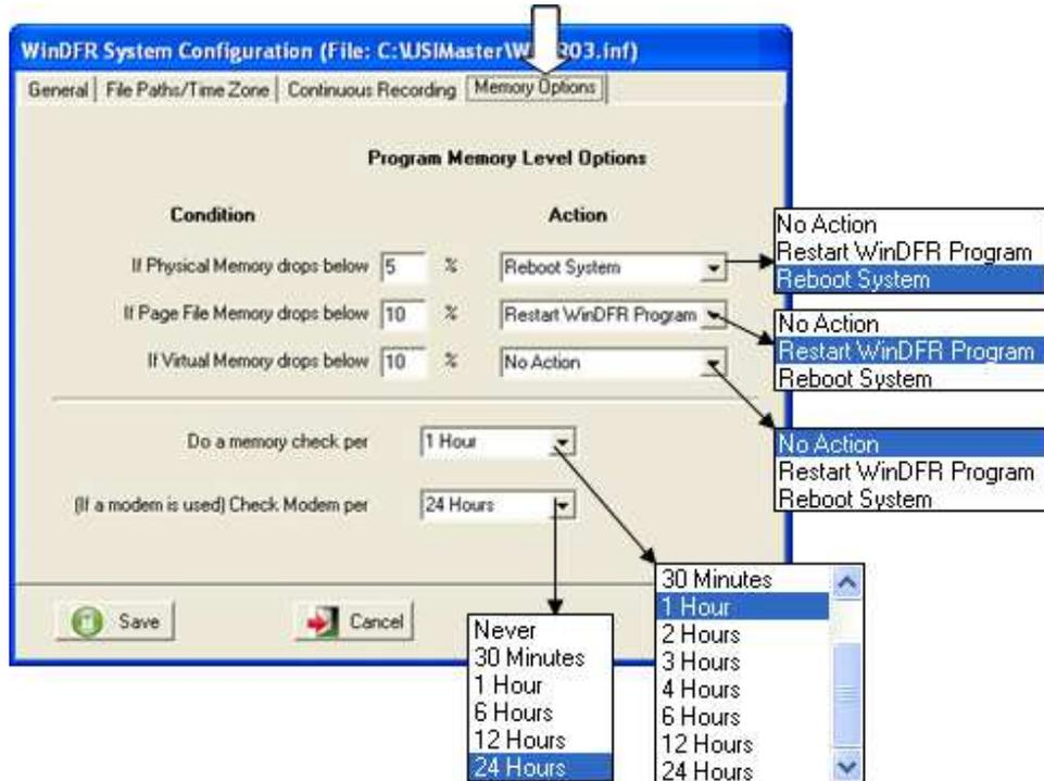
**Figure 2-59 WinDFR® Configuration Screen – Memory Options Tab**
