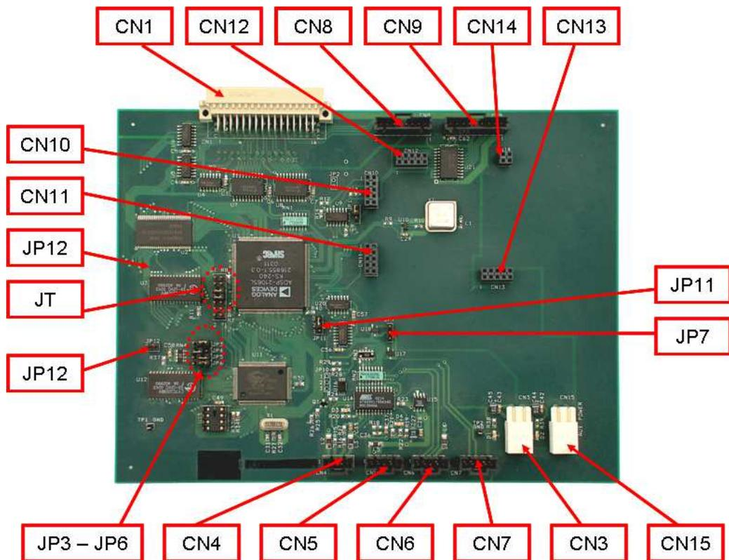
**Figure A.1.1-1 DSP Board (First Generation) – Top Side**
