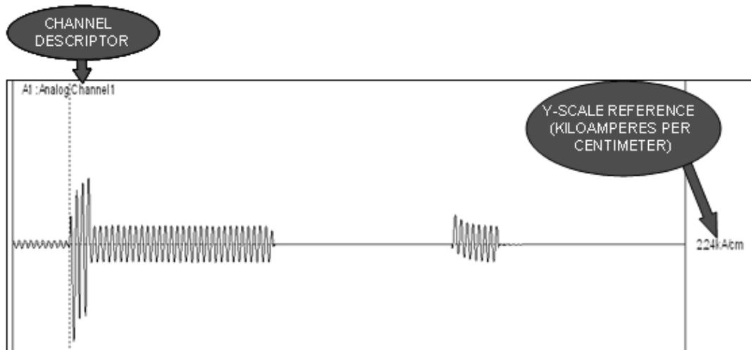
**Figure 2-38 Y-Scale – Channel Full-Scale – Unit/Centimeter – Sample Printout**
