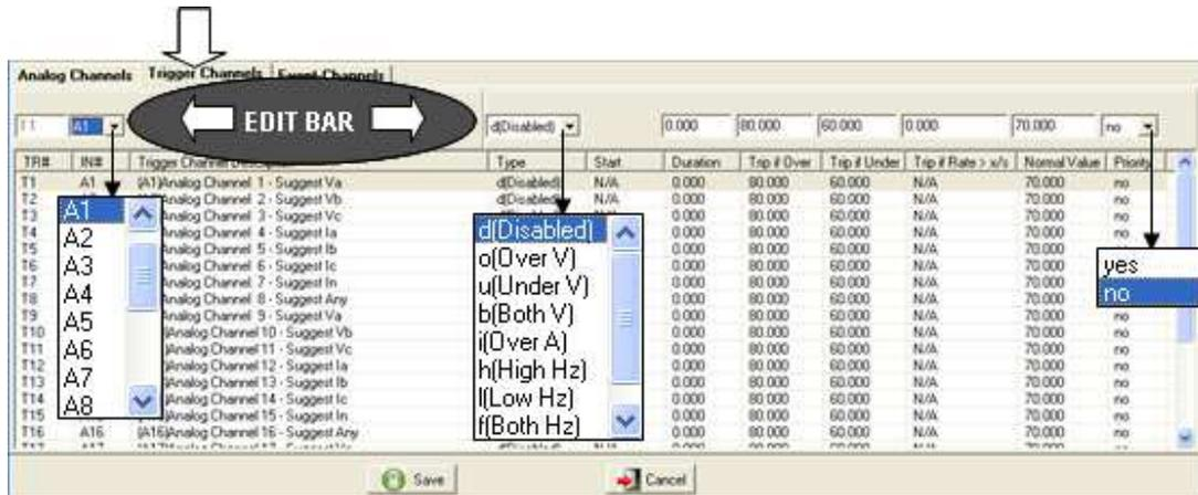
**Figure 2-74 Calibration Record Trigger Channels –Version 093a**
