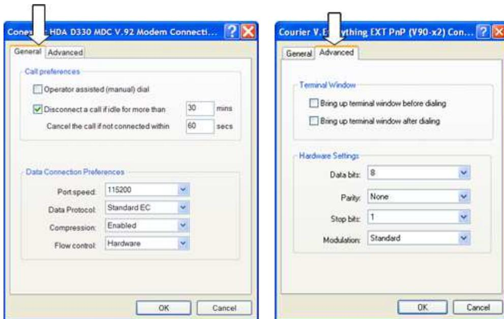
**Figure 2-8 Configure Modem**
