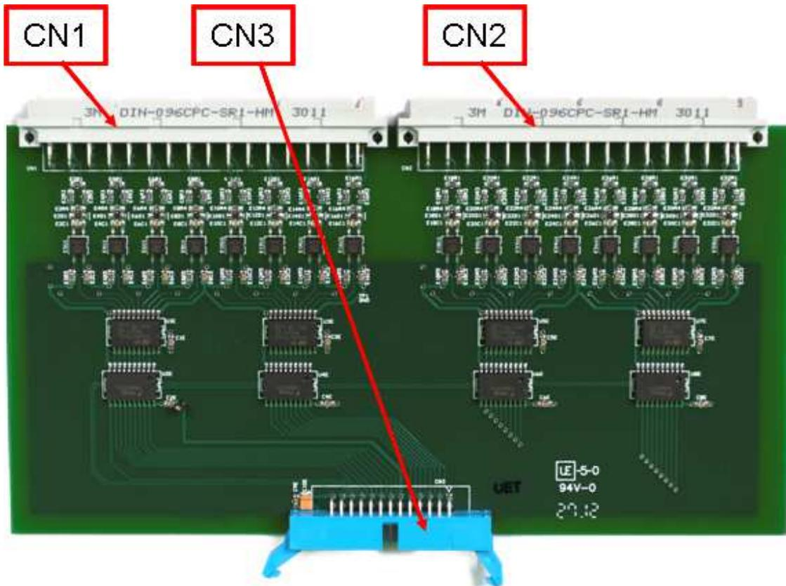
**Figure A.1.13 Low-Voltage Digital Board (First Generation)**
