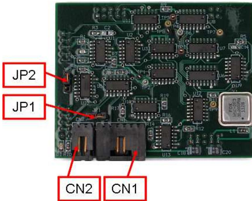
**Figure A.1.4-1 Common Board (Second Generation) – Top Side**
