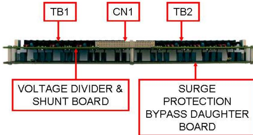
**Figure A.1.7-2 High-Voltage Analog Board (Dual Board Version) – Front Side**
