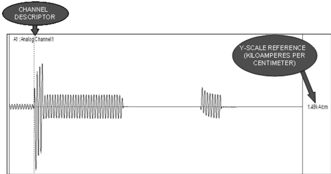
**Figure 2-37 Y-Scale – Optimized – Unit/Centimeter – Sample Printout**
