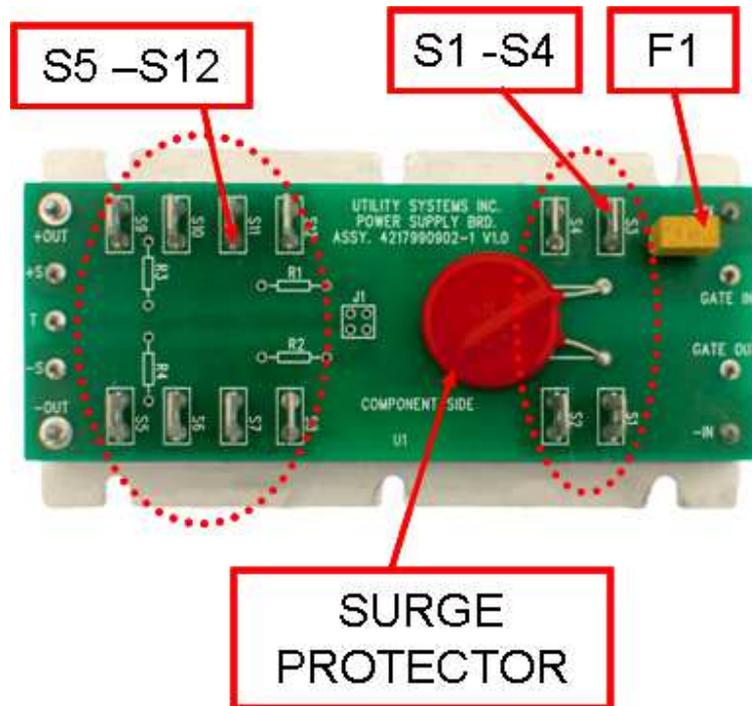
**Figure A.1.15-2 DC-to-DC Converter module**
