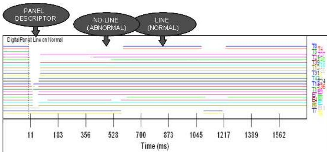
**Figure 2-42 Sequence of Events/Triggers – Line on Normal – Sample Printout**
