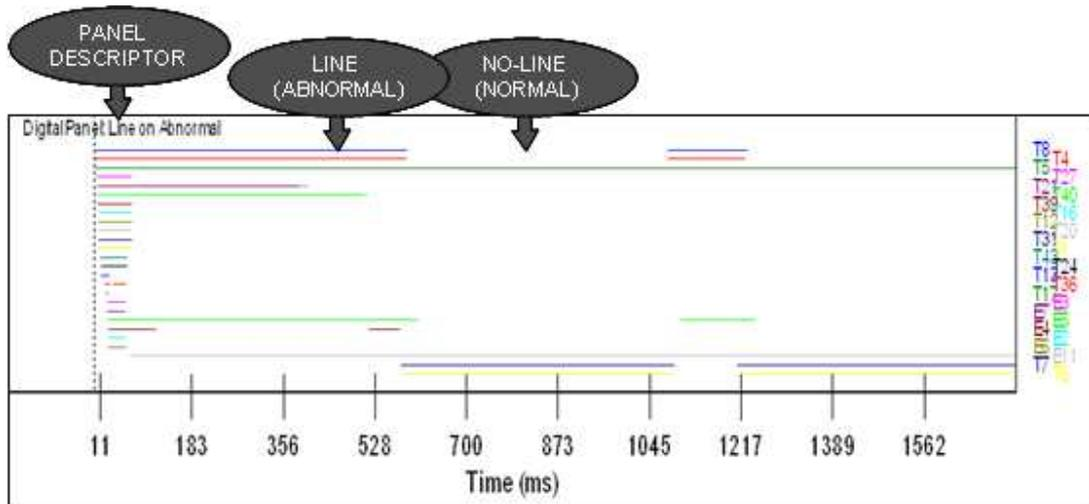
**Figure 2-41 Sequence of Events/Triggers – Line on Abnormal – Sample Printout**
