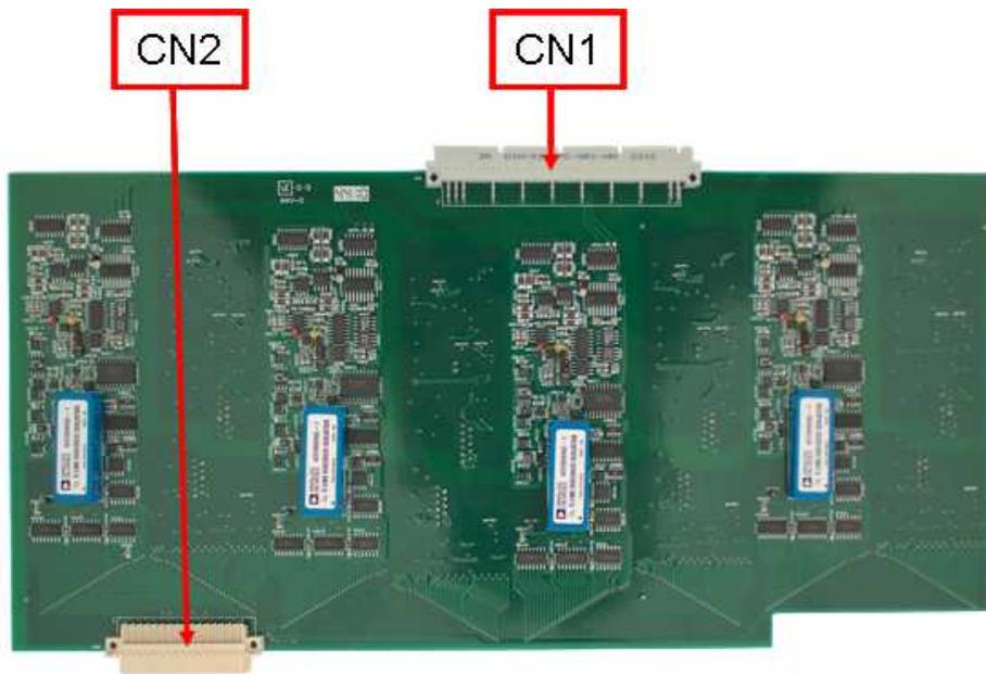
**Figure A.1.9-1 Low-Voltage Analog Board (First Generation) – Top Side**
