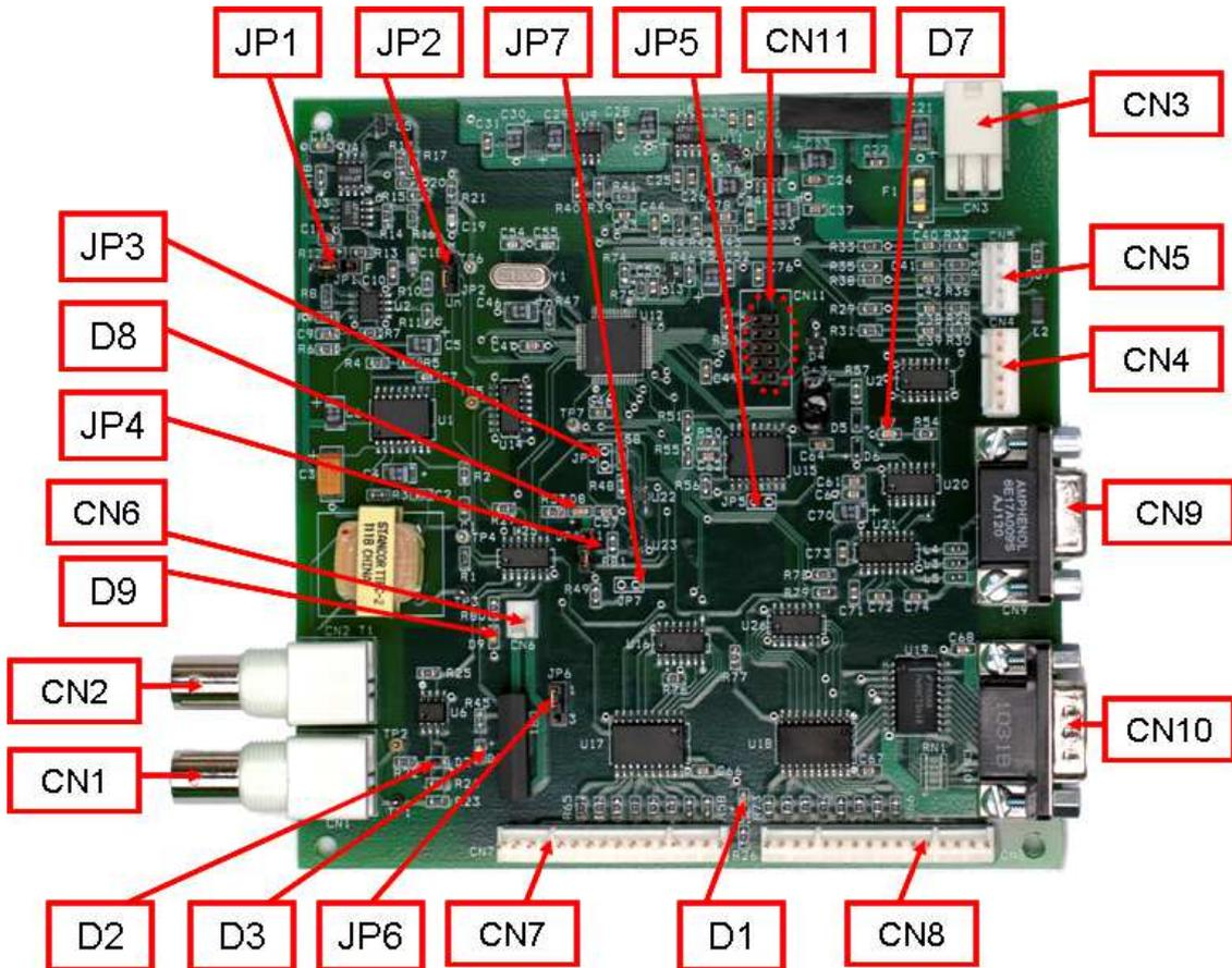
**Figure A.1.6 I/O-IRIG Board (Second Generation)**
