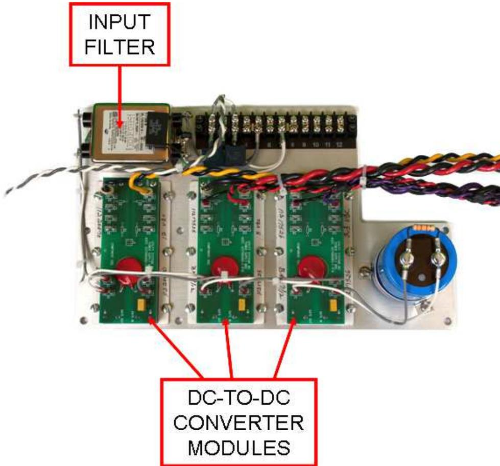
**Figure A.1.15-1 Power Supply Assembly**
