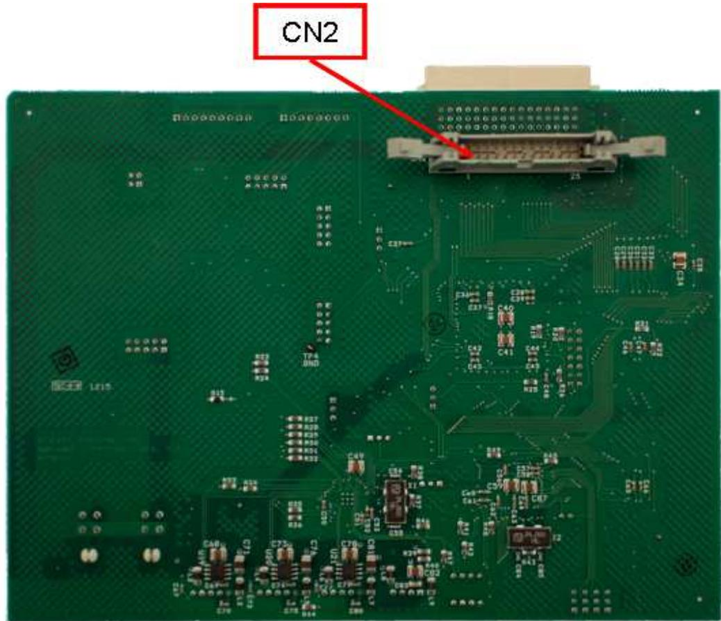
**Figure A.1.2-2 DSP Board (Second Generation) – Bottom Side**
