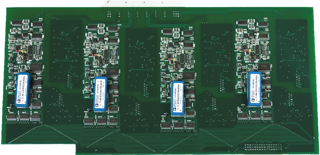
**Figure A.1.9-2 Low-Voltage Analog Board (First Generation) – Bottom Side**
