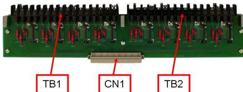
**Figure A.1.7-1 High-Voltage Analog Board (Dual Board Version) – Top Side**
