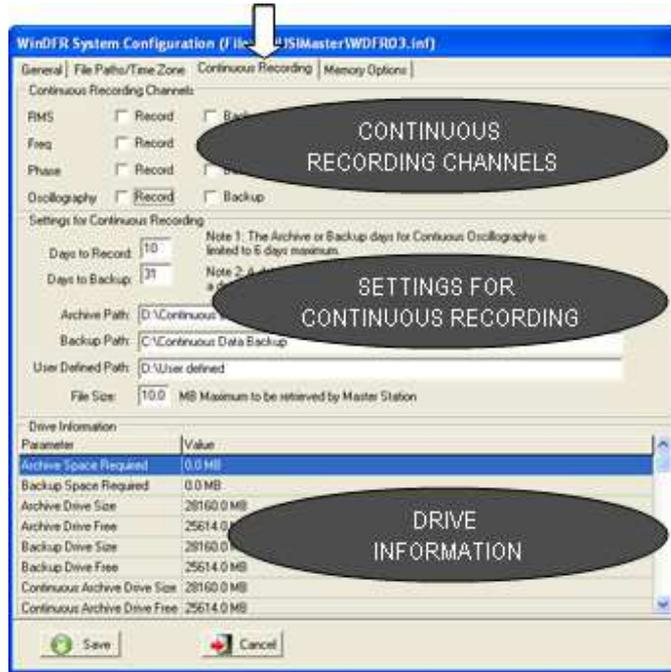
**Figure 2-55 WinDFR Configuration Screen - Continuous Recording Tab**
