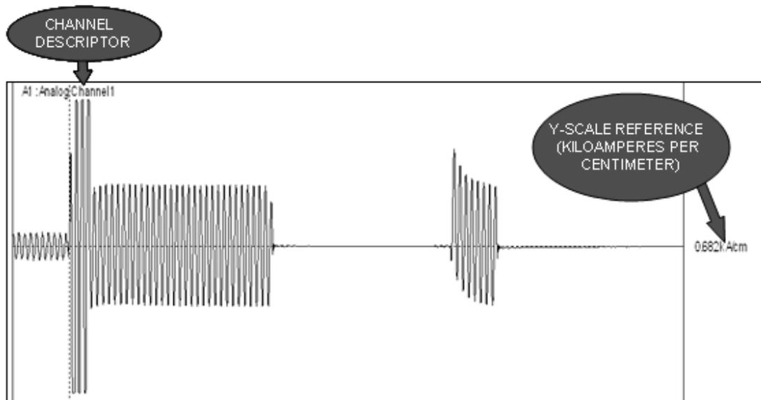
**Figure 2-40 Y-Scale - User Selected – Unit/Centimeter – Sample Printout**
