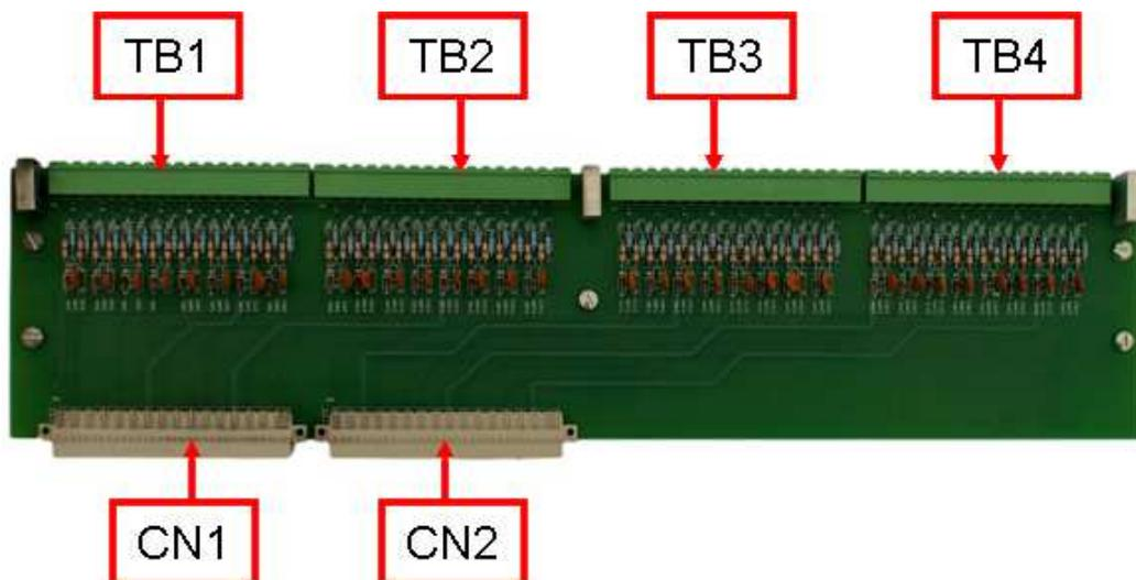
**Figure A.1.11-1 High-Voltage Digital Board (Dual Board Assembly) – Top Side**
