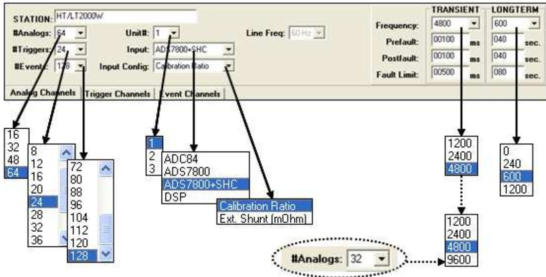
**Figure 2-72 Calibration Record Station Header –Version 093a**
