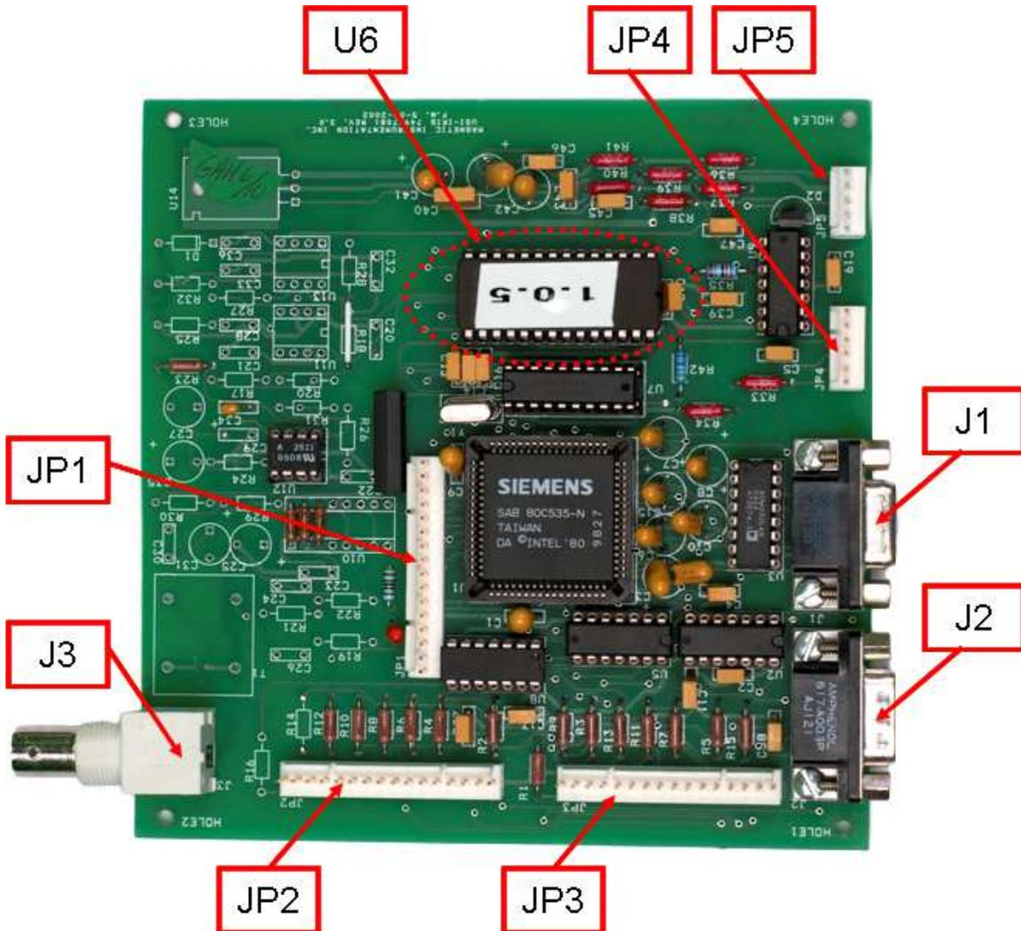
**Figure A.1.5-2 Input/Output Board (First Generation) – Unmodulated**
