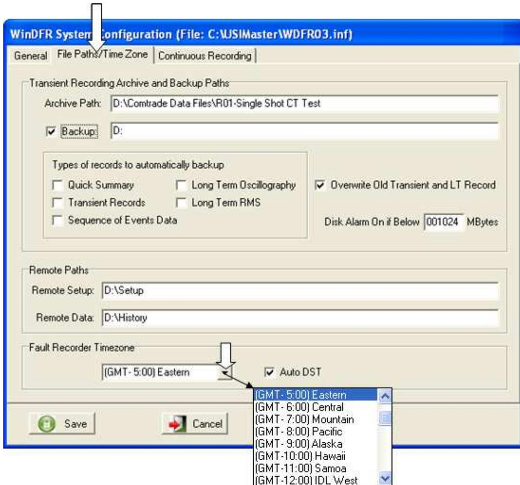
**Figure 2-53 WinDFR Configuration Screen - File Paths/Time Zone Tab**
