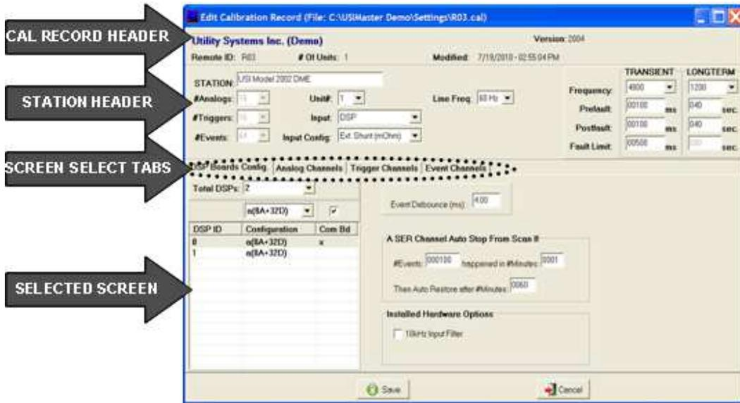
**Figure 2-60 Calibration Record Screen**
