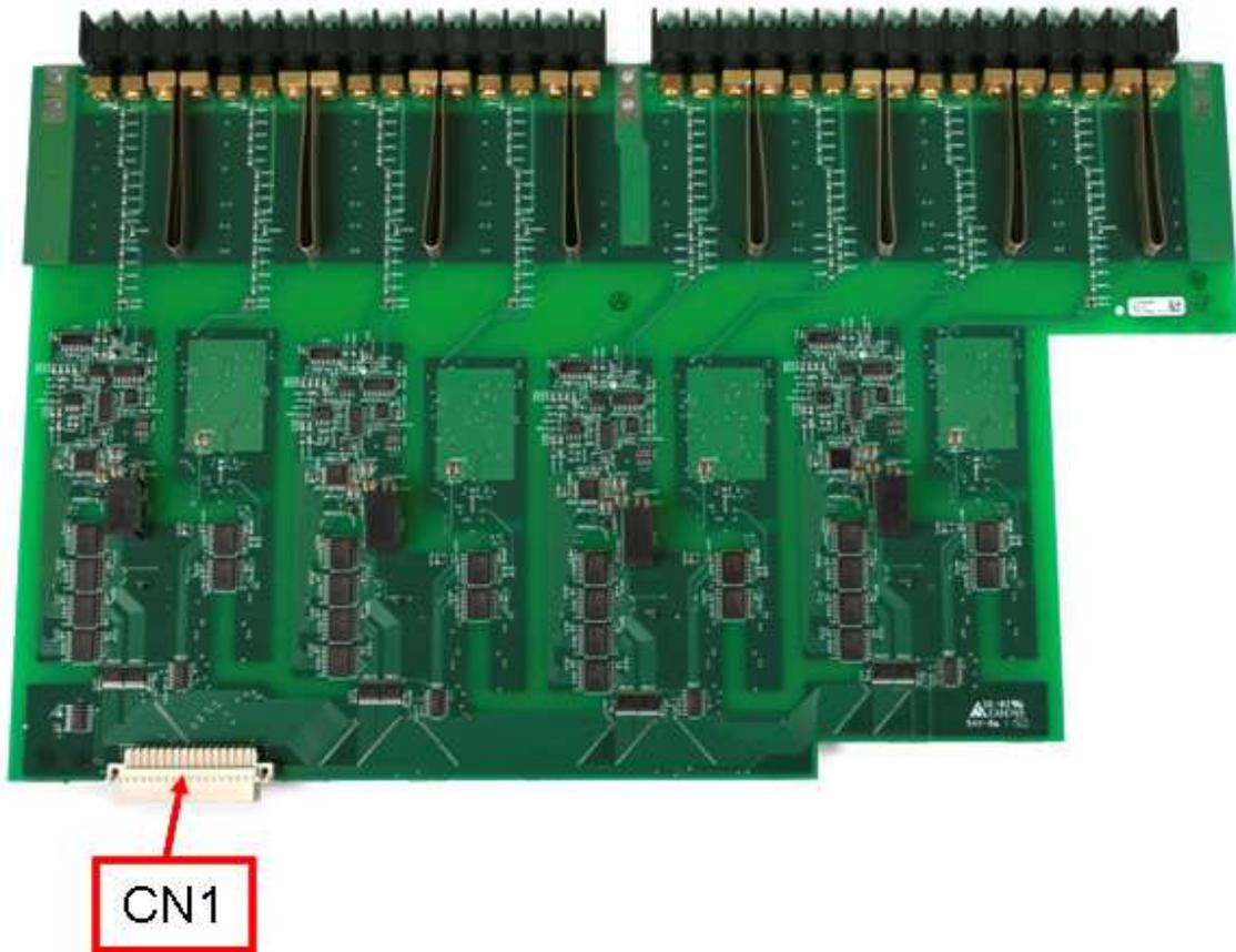
**Figure A.1.10 Analog Board (Second Generation)**
